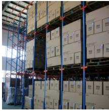
Drive-in and drive-through pallet rack are storage rack configurations that allow the forklift to drive directly into the lane of stacked rows. Drive-in Pallet Racking produces efficiencies through decreasing section launching as well as unloading occasions, however permitting higher entry when compared with block-stacking. Placement pallets upon front-to-back bed rails enables series to become piled following to one another properly as well as effectively
